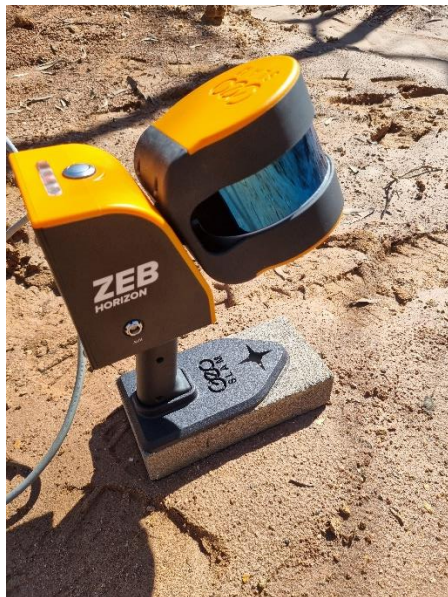
Figure 1 GeoSLAM ZEB Horizon on a control point
