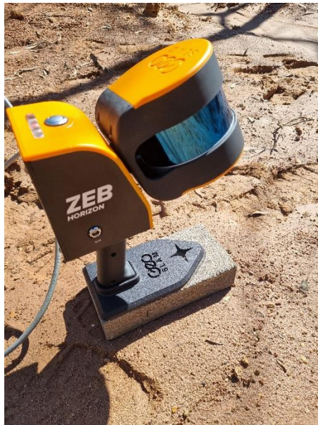
Figure 1 GeoSLAM ZEB Horizon on a control point
