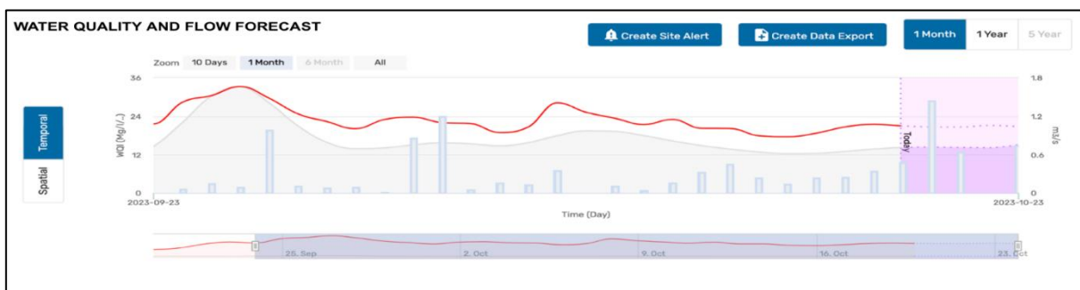
Figure 2. The Dashboard Display showing Rainfall, Flow and Nitrate Concentrations Simulated for the River Colne with a Three Day Forecast in pink.
