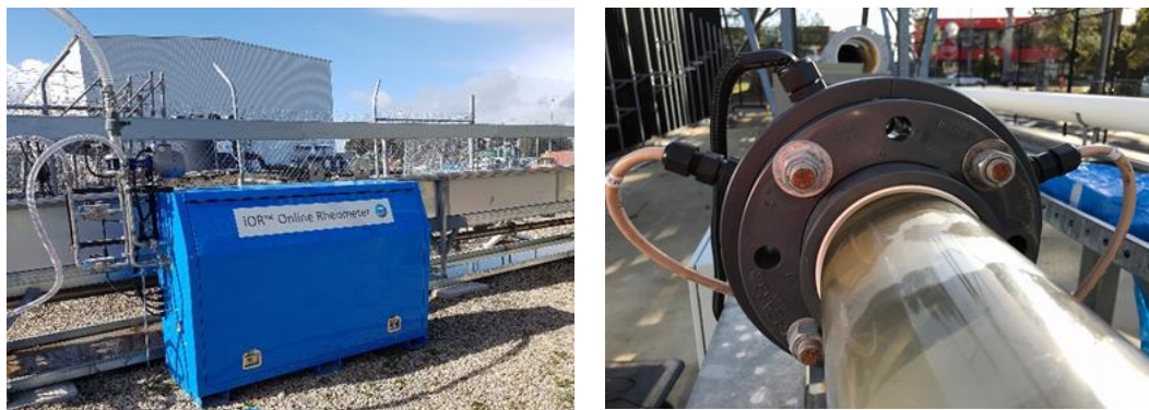
Figure 2. The CSIRO developed (a) intelligent Online Rheometer (b) Bed Load Detector integrated into a pipeline
