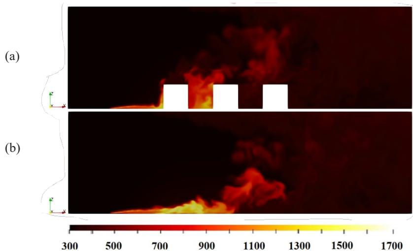
**Figure 4.** The contour of temperature distribution for the case with  $U= 6\text{ m/s}$  and  $I= 10\text{ MW/m}$ :
