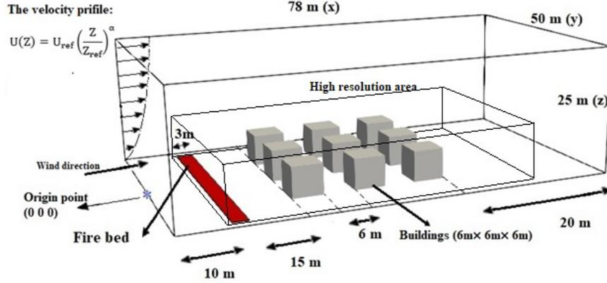
**Figure 1.** Schematic of computational domain and the location of the buildings
