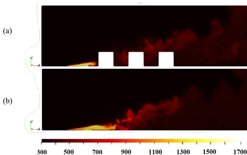
**Figure 5.** The contour of temperature distribution for the case with  $U= 12\text{ m/s}$  and  $I= 10\text{ MW/m}$ :
