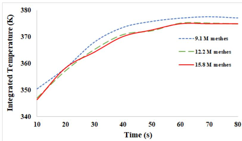
**Figure 3.** Comparison of the average temperature of the domain versus time for three different grids number
