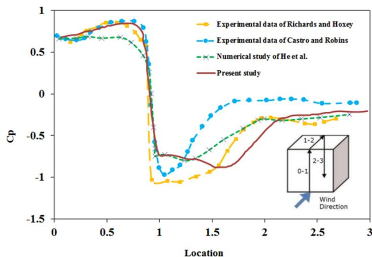
**Figure 2.** Comparison of the mean pressure coefficient for the experimental studies of Richards and Hoxey (2012) and Castro and Robin (1977) and numerical simulation of He et al. (2011)
