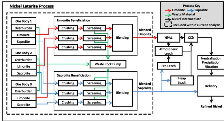
Figure 1: Schematics of nickel laterite production system.
