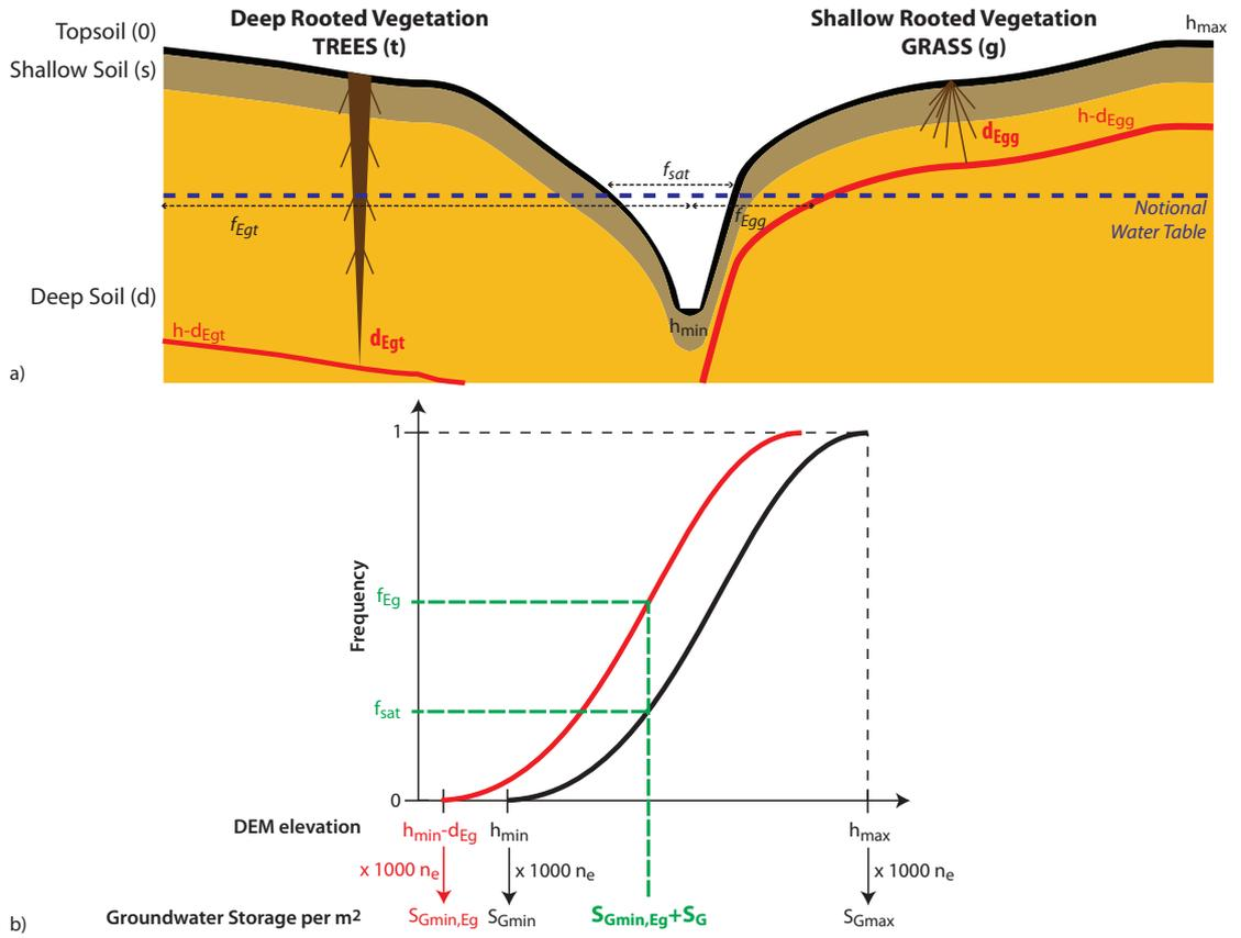
**Figure 1.** a) AWRA-L conceptual cross-section for a grid cell with 50 % deep rooted vegetation and 50 % shallow rooted vegetation. b) Elevation hypsometric curves
