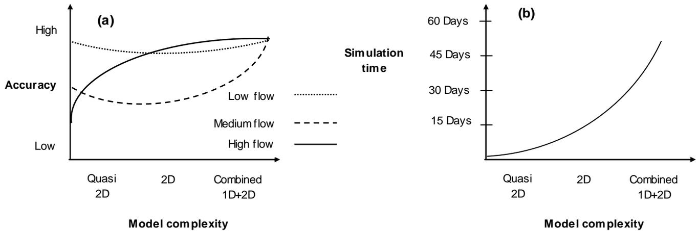
**Figure 4.** Conceptualised relationships between complexity of the floodplain model forms MIKE 11 (Quasi 2D), MIKE 21 (2D) and MIKE FLOOD (Combined 1D+2D) and accuracy of the simulated inundation areas (4a), and simulation times (4b). (Results from model implementations on a Intel (R) dual core™ PC with 2.13 GHz processor speed and 3.25 GB RAM for study area of about 337 km<sup>2</sup>)
