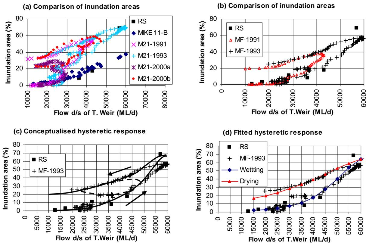
**Figure 3.** (a–b) Comparison of the inundation area estimates from remote sensing analysis (RS) with results from MIKE 21 (M21) and MIKE FLOOD (MF) hydraulic models (d/s: downstream; T.Weir: Torrumbarry Weir); (c) conceptualised hysteresis inundation response relationship between floodplain inundation area versus flow in the Murray; and (d) fitted parametric forms of the wetting and drying phases of the hysteresis KPF flood inundation response to variation of flow in the Murray.
