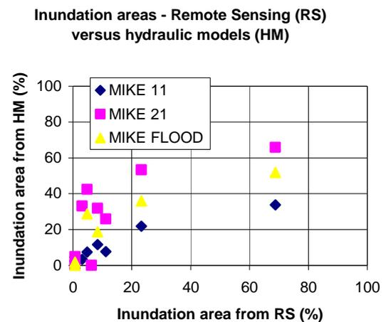
**Figure 2.** Comparison of inundation area estimates from hydraulic models and results from the remote sensing analysis.
