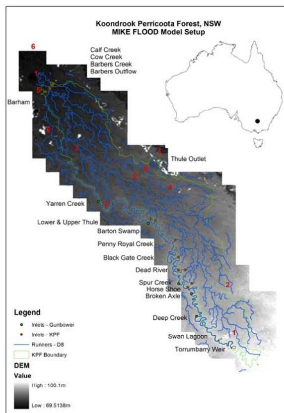
**Figure 1.** Location map and the KPF floodplain model developed from LiDAR DEM at 1 m grid cell resolution. Six runners (1–1 to 6–6) were used to define 809 runner cross-sections of 200 m width at an average spacing of 226 m, as well as eight KPF inlets and five KPF outlets.
