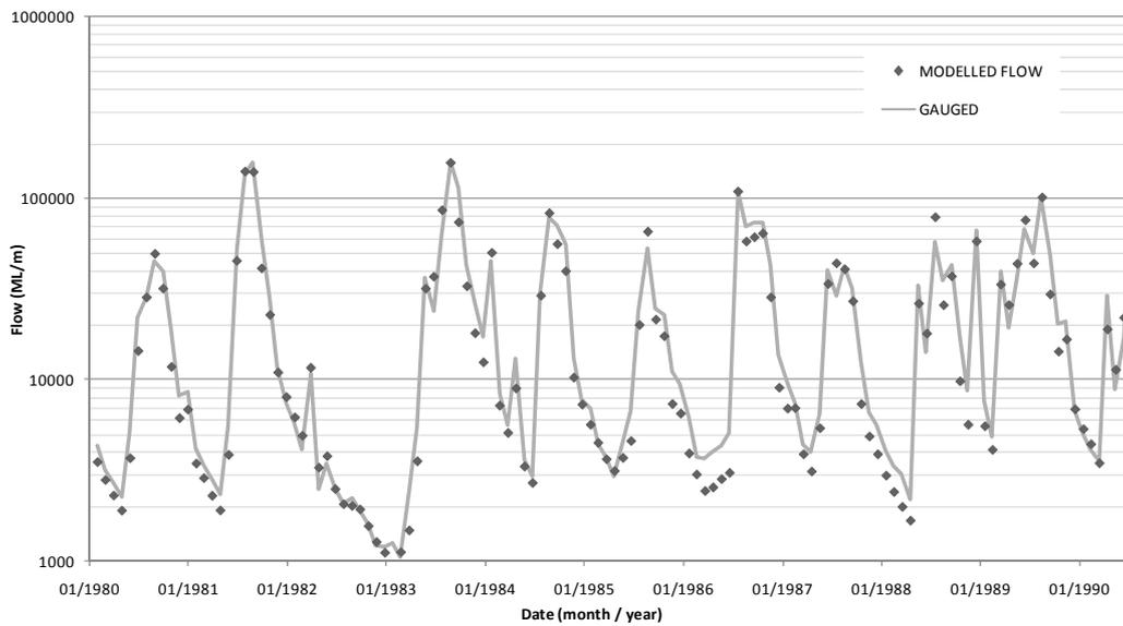
**Figure 3:** Monthly flow (modelled and observed) ( $\alpha=160$ ,  $\beta=1$ ,  $\gamma=1$ ,  $P=1$ ,  $D=0$ ,  $L=0$ ) [note log scale].
