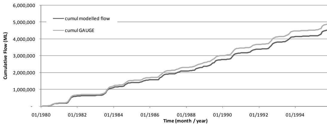
**Figure 4:** Cumulative flow (modelled and observed) ( $\alpha=160$ ,  $\beta=1$ ,  $\gamma=1$ ,  $P=1$ ,  $D=0$ ,  $L=0$ ).
