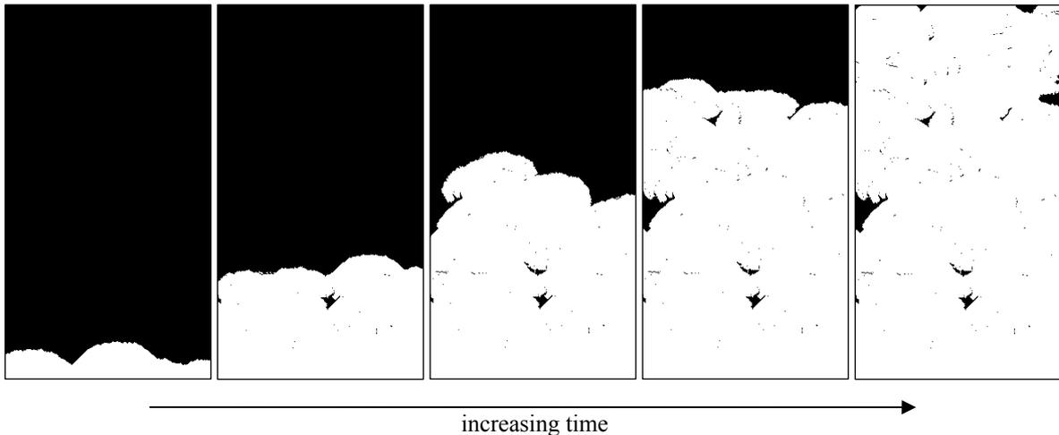
**Figure 3.** A time slice of a segment of the simulation output depicting the cold spray deposition process (each image has dimensions  $470 \times 255 \mu\text{m}$ ). The dark areas correspond to voids whilst the white areas correspond to those containing copper.
