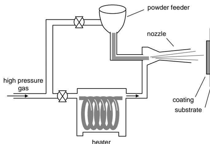
**Figure 1.** Schematic diagram of a cold spray deposition system.
