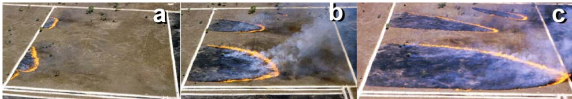
Figure 2. Oblique aerial photos 3 experimental fires lit simultaneously (from left to right: 100-m ignition, 50-m ignition, and point ignition). (a) 40 s since ignition: The 50 m and 100 m fires have spread a similar distance; the point ignition is barely discernible. (b) 100 s since ignition: The 100-m fire is spreading faster than the 50-m fire; the point ignition fire is now visible. (c) 160 s since ignition: The 100-m fire has reached the end of the block; the 50 m and the point ignition fires are now spreading at roughly the same speed. (Source: Cheney and Gould (1995))
