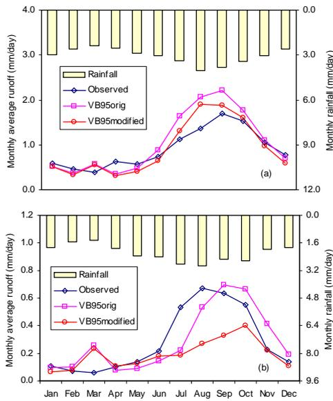
**Figure 4.** Simulated (using both the original VB95 and the modified model) and observed seasonality in runoff for (a) the Cotter River (410730) and (b) Tarcutta Creek (410047). The seasonal rainfall distribution is also shown.
