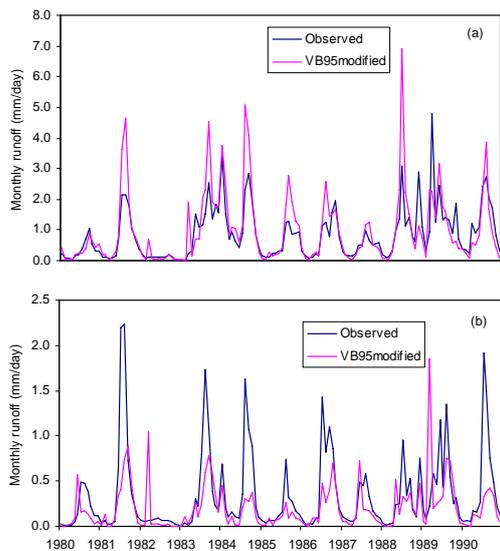
**Figure 8.** Simulated (modified VB95) and observed monthly runoffs for (a) the Cotter River (410730) and (b) Tarcutta Creek (410047)
