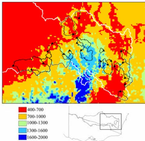
**Figure 1.** Gauged unregulated catchments in the mid- and upper-Murrumbidgee catchment. The mean annual rainfall (mm) is shown.
