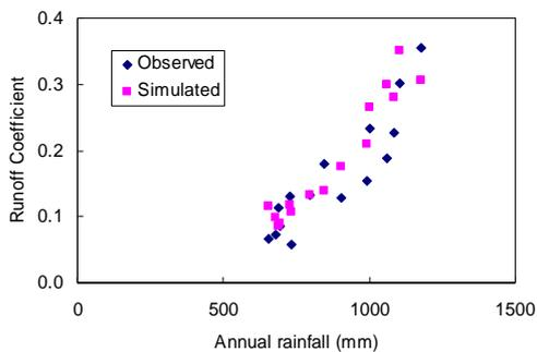
**Figure 2.** Simulated and observed runoff coefficients for 15 catchments in the mid to upper Murrumbidgee River Basin
