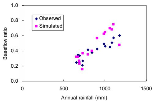
**Figure 7.** Simulated (modified VB95) and observed baseflow index for 15 catchments in the mid to upper Murrumbidgee River Basin
