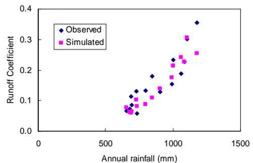
**Figure 6.** Simulated (modified VB95) and observed runoff coefficients for 15 catchments in the mid to upper Murrumbidgee River Basin
