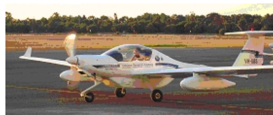
Figure 6. The Diamond ECO-Dimona aircraft with PLMR mounted under the fuselage, and thermal imager, digital camera and NDVI scanner in an underwing pod.
