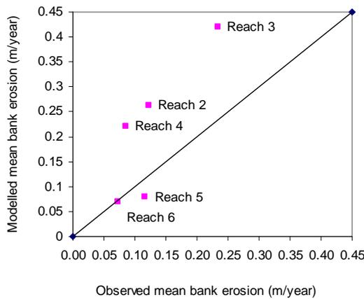
**Figure 2.** 1:1 plot of observed versus modelled mean bank erosion rate by the river reaches.
