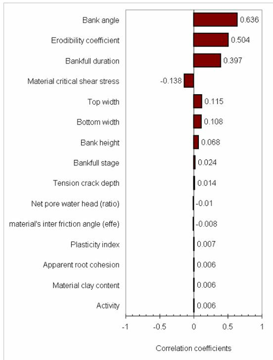
**Figure 4.** Correlation Tornado plot between the inputs and the bank erosion rate for the reach two. Longer bars at the top show the most sensitive variables.
