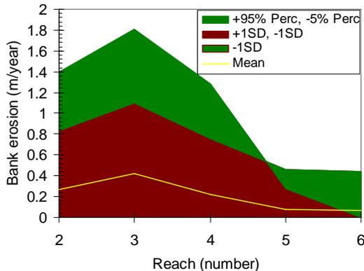
**Figure 3.** Summary plot showing the bands of the bank erosion at the reaches ( $BE_s$  at  $\pm 1$  standard deviation, 95<sup>th</sup> and 5<sup>th</sup> (always zero) percentile values).
