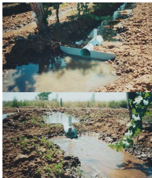
Figure 2. Circular flume used for furrow inflow determination, note hydraulic jump in the bottom picture.
