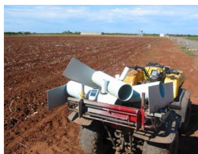
Figure 3. GPS for measuring advance distance to calculate infiltration characteristics and portable circular flumes.
