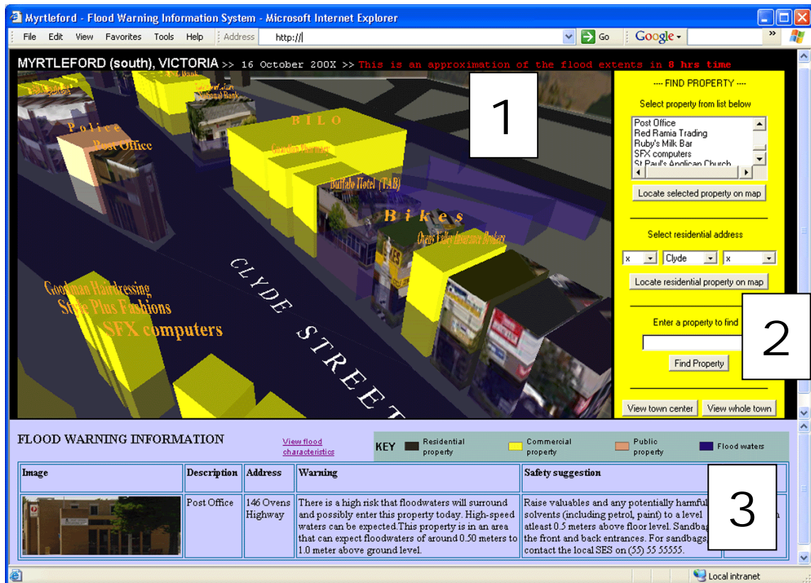
Figure 1. A screen grab of the prototype FWIS interface. Numbers in white boxes refer to: 1) The 3D map displayed by the Flood Warning tool; 2) the Find Property tool; 3) Information displayed by the Safety Information.
