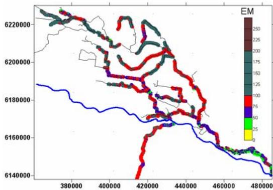
**Figure 2.** EM31 Map of surveyed channels in the Murrumbidgee Irrigation Area (MIA)
