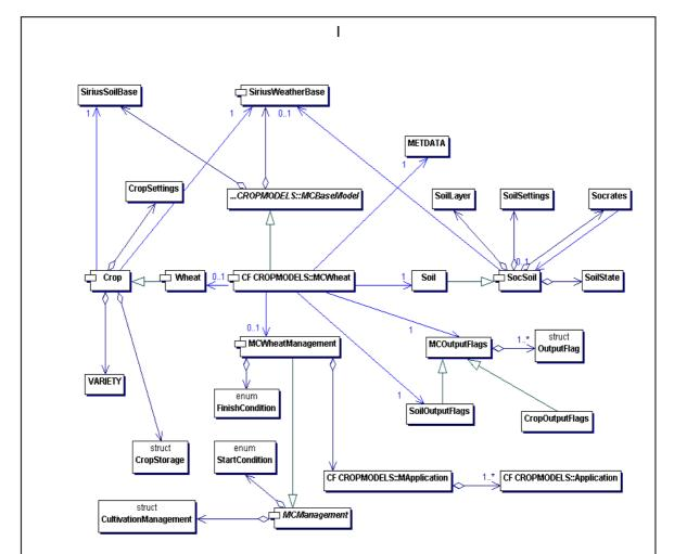
Figure 2. An outline of the class diagram of the MCWheat, the seasonal model for wheat in the LUCI framework model. This is a seasonal model which processes the crop, soil, METDATA and management day step models and co-ordinates the transfer of required information from one model to another.
