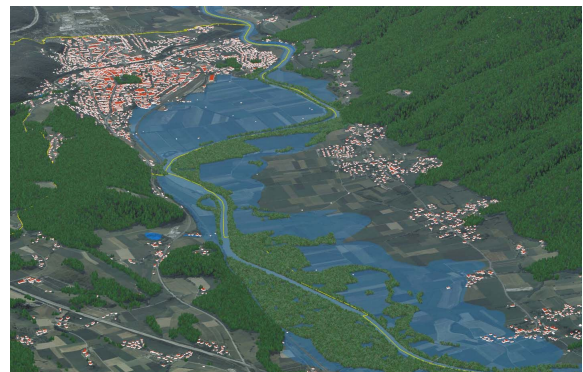
Figure 1. Digital flood risk map of the river Drau (Carinthia/Austria) resulting from a 2D-CFD-simulation based on a high resolution ALS-DTM
