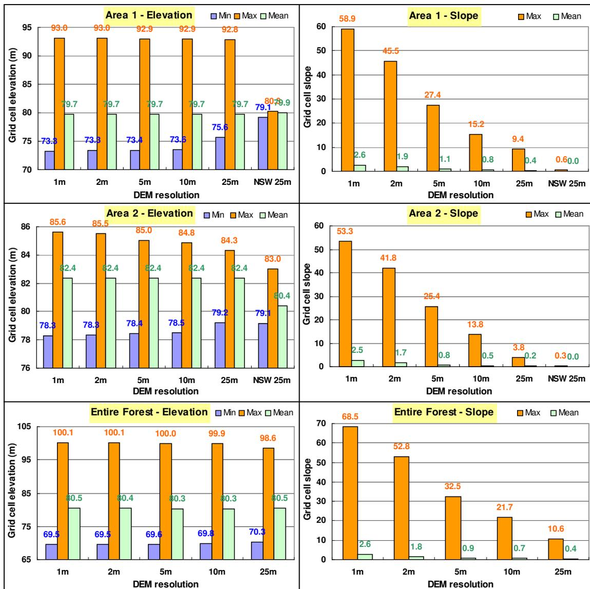
Figure 2. Variation in minimum, maximum and mean grid cell elevation and slope for 1m, 2m, 5m, 10m, 25m LiDAR and 25m NSW DEM for Area 1, Area 2 and the entire forest
