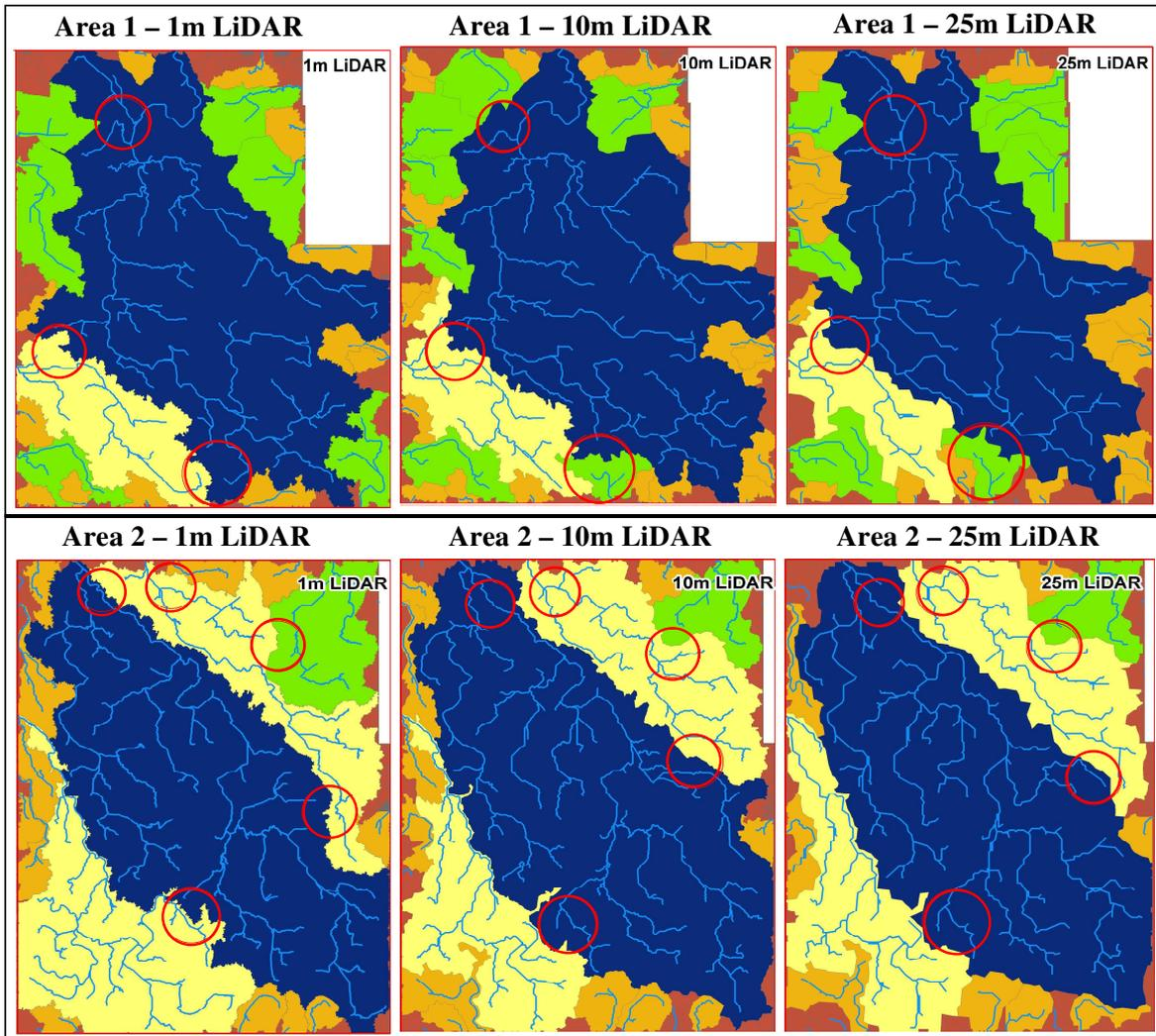
Figure 3. Stream network and watersheds for Area 1 and Area 2 derived from different resolution DEM's
