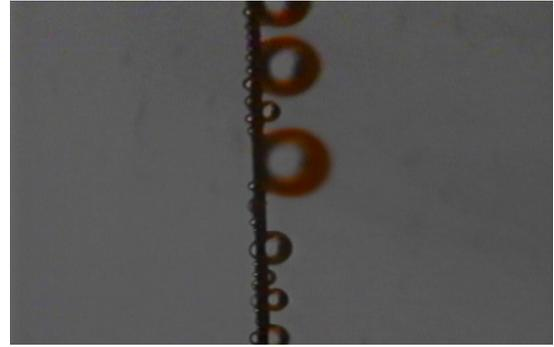
**Figure 4.** Clamshell droplets on  $28 \mu\text{m}$  SS fibre –  $V=6\text{m/s}$ , flow is left to right.
