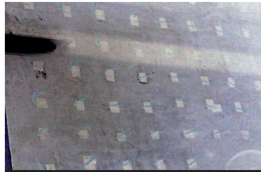
Figure 3 Recirculation zone detected by the tuft method on the horizontal top wall above the rotating blades.
