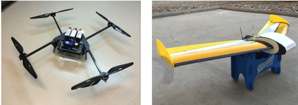
Figure 1. (left) a custom-designed quadcopter with a sensor load of just over 1 kg; and (right) the QuestUAV system. The UAVs carry a common sensor package comprising a SONY NEX-7 20MP digital camera, an Optris-Pi450 broadband thermal camera (7.5 to 13 \mu\text{m} ) and a Tetracam MiniMCA that records 6 unique spectral bands across the VNIR (i.e. 490, 560, 665, 705, 740, 865 nm center wavelengths) that is configured to match those on Sentinel-2, a new satellite system launched in June 2015.
