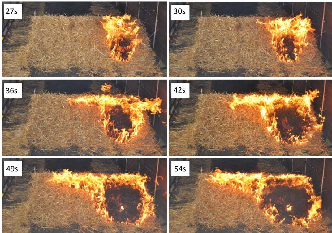
**Figure 4.** Fire spread on the leeward slope of the hill during Test 4 looking upwind. The time since fire ignition is indicated in each frame. This test was carried out with configuration 2 of the hill and with a wind velocity of 3 m/s.
