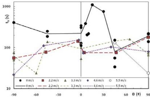
**Figure 3.** Duration  $t_b$  of combustion for EB as a function of orientation angle and flow velocity.
