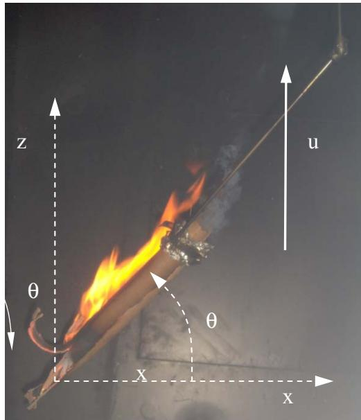
**Figure 1.** Definition of the orientation angle  $\theta$  between the particle axis and the horizontal direction. The flow velocity is vertical from the bottom to the top of the picture.
