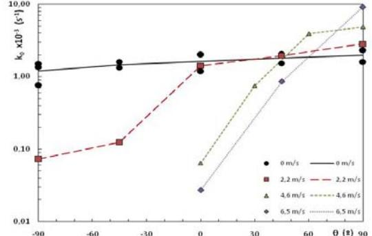
**Figure 6.** Exponential mass loss coefficient  $k_o$  variation during the entire combustion process for PC as a function of orientation angle and flow velocity.
