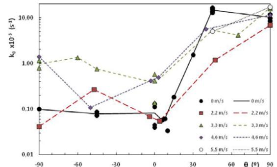
**Figure 4.** Exponential mass loss coefficient  $k_o$  variation during the entire combustion process for EB as a function of orientation angle and flow velocity.
