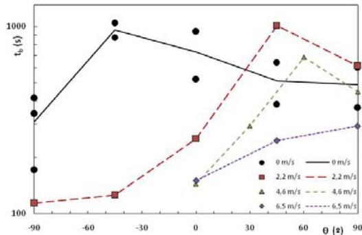
**Figure 5.** Duration  $t_b$  of SC for PC as a function of orientation angle and flow velocity.
