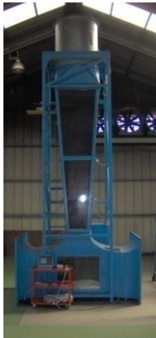
**Figure 2.** The Vertical Combustion Tunnel (TCV) of the Fire Laboratory of ADAI.
