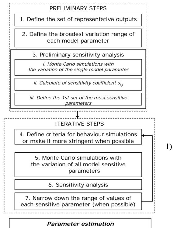
**Figure 2.** Flow chart of the proposed procedure for parameter estimation.
