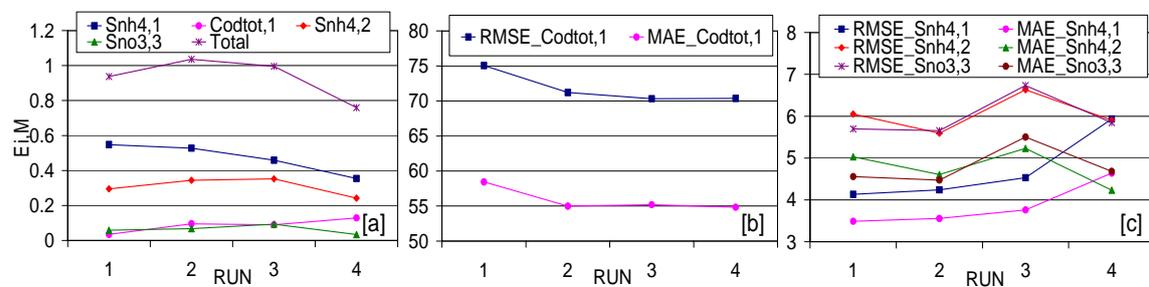
Figure 4. [a] Values of the efficiency of each representative variable *i*th which correspond to the maximum value of the sum of the efficiencies for the four variables ( $E_{i,M}$ ); [b] RMSE and MAE of CODtot,1; [c] RMSE and MAE of Snh4 in the section 1 and 2 and Sno3,3.
