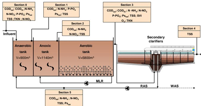
Figure 1. Flow sheet of WWTP with locations of sampling points.
