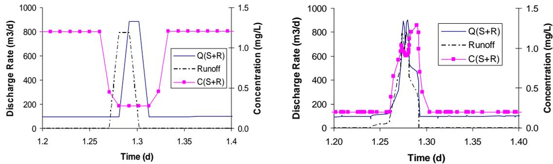
**Fig. 4.** Simulated temporal patterns of discharge and concentrations of NO<sub>3</sub> (left) and phosphate (right) during a complex rainfall event in the Montagu catchment that led to runoff.
