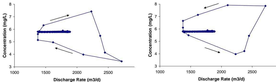
**Fig. 3.** Patterns of  $C(Q)$  simulated for the Rusjan et al (2008) August II-5 rainfall event assuming peak concentrations preceded (left) or followed (right) peak discharge. The direction of hysteresis is indicated by arrows. Runoff method A was used.
