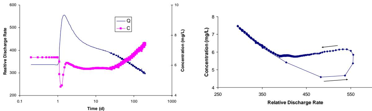
**Fig. 5.** A rainfall runoff event simulated with three water sources with contrasting concentrations. This scenario is akin to type A3 as described Evans and Davies (1998), i.e. ground-water concentration ( $C_G$ ) > soil water concentration ( $C_{SW}$ ) > event concentration ( $C_{SE}$ ). The direction of hysteresis is indicated by arrows.
