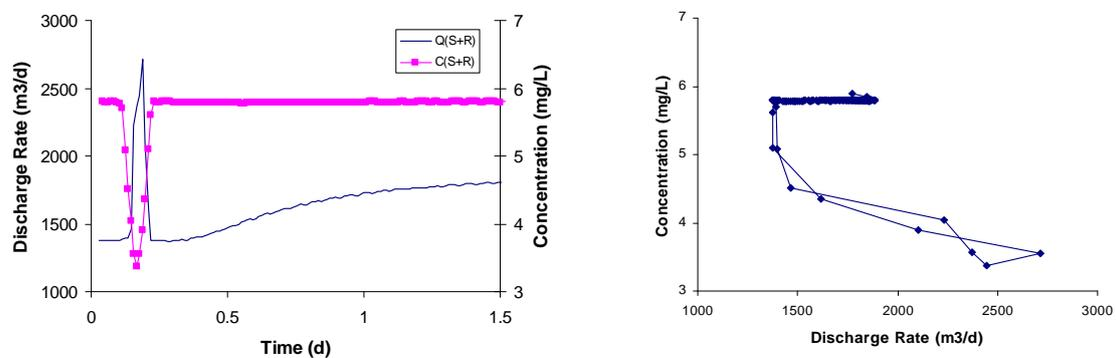
**Fig. 2.** Patterns of  $C(Q)$  simulated for the Rusjan *et al.* (2008) August II-5 rainfall event in Slovenia. Significant runoff occurred during this event (observed and simulated). Simulated flow (left) shows the separate influence on flow of runoff that lasted a few hours and longer-term seepage at an increased rate due to infiltration. Runoff method A was used.
