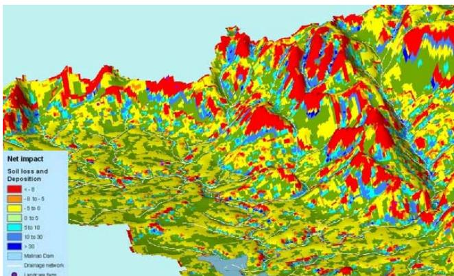
Figure 3. Areas of erosion and deposition with current land use (Runoff flow = 100).
