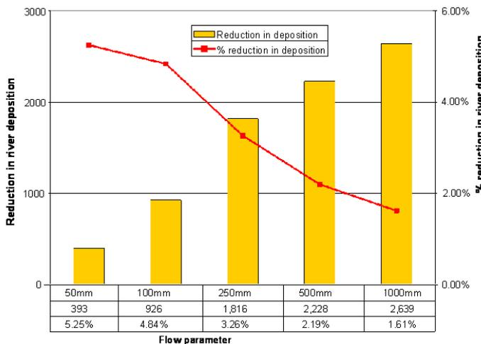
**Figure 5.** Impacts of land use change of sediment deposited in drainage network
