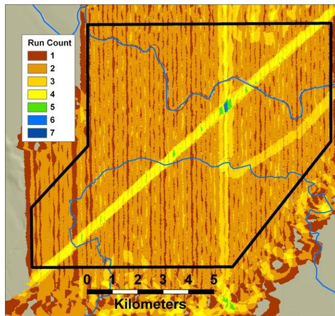
**Figure 2: Flight run geometry showing extent of overlap in LiDAR survey data.**
