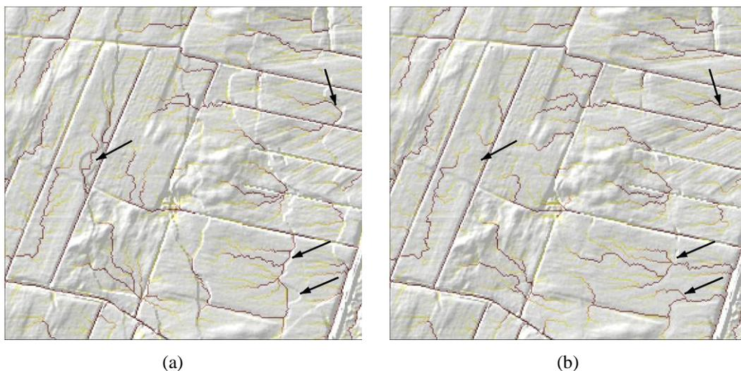
**Figure 5: An example of improvement to flow patterns resulting from DEM height adjustments (a) flow patterns in merged grid of unadjusted DEMs (b) flow patterns in merged grid of adjusted DEMs. Arrows indicate flow lines that were artificially constrained by edge stepping in the original DEM.**
