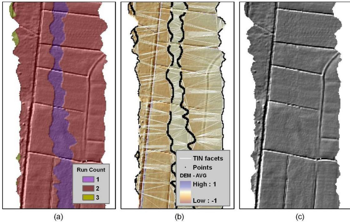
**Figure 4: Height corrections steps for a single run: (a) Determine edges using run count information and determine spatially averaged heights at each edge (b) Generate adjustment points along all edges (black dots) and remove those that occur near sharp landscape features then construct a TIN lattice (white lines) to interpolate between points. (c) Use the TIN structure to determine adjustments for DEM and apply.**
