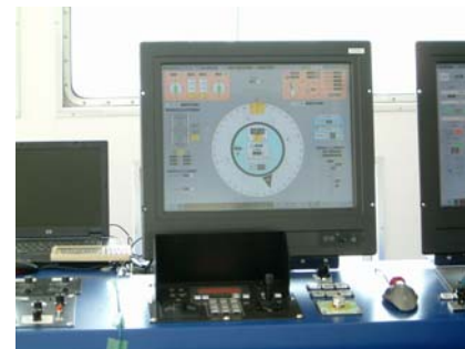
Figure 5. Control Station (Master Panel)
