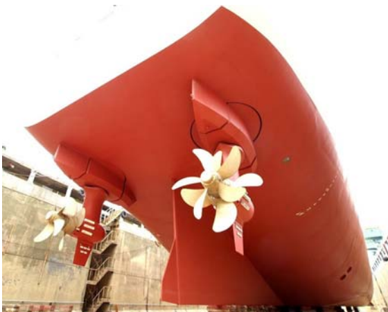
Figure.2 Outline of Azimuth Propellers
