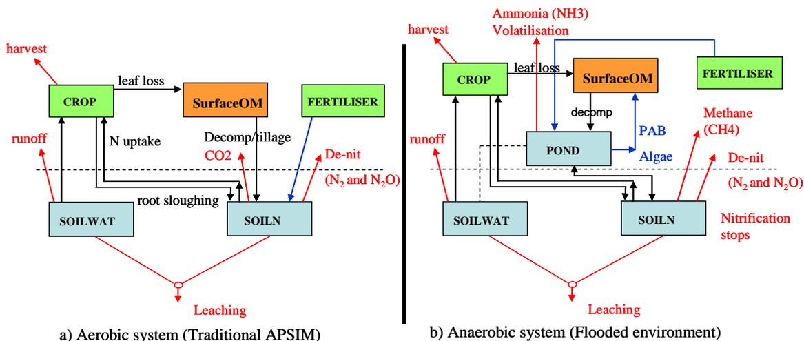
**Figure 1.** Conceptual structure of APSIM module communications and C&N loss (red) and gain (blue) mechanisms in: a) traditional aerobic systems; and b) flooded systems. The black dotted line represents the soil surface.
