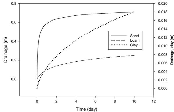
**Figure 5.** Cumulative drainage with time for sand, loam and clay form an initially saturated domain with free drainage on the bottom boundary.
