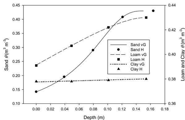
**Figure 6.** Comparison of water content profiles in the centre of the bed form simulation (H) with estimates using equation (5) (vG).
