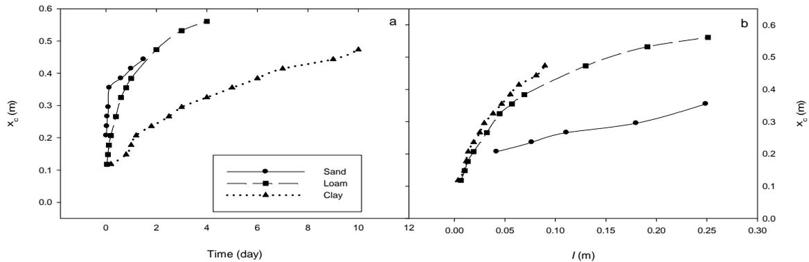
**Figure 3.** Washout distance ( $X_c$ ) with a) time and b) cumulative infiltration ( $I$ ) for sand, loam and clay soils.
