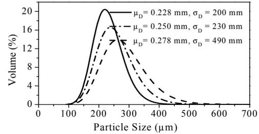
**Figure 2.** Particle size distribution of mixed-sized grain bed with the principle of logarithmic normal distribution.
