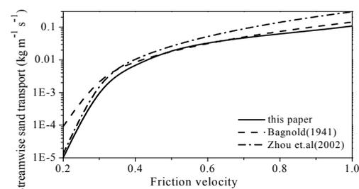
**Figure 9.** The streamwise sand transport at friction velocity
