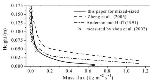
**Figure 5.** The mass flux profiles at steady state
