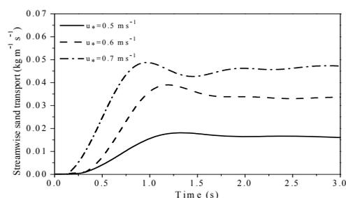
**Figure 7.** Evolution of the streamwise sand transport at different friction velocity.
