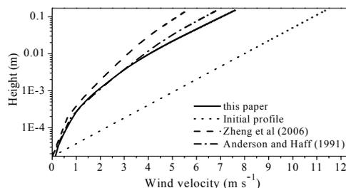
**Figure 6.** The wind profiles at steady state
