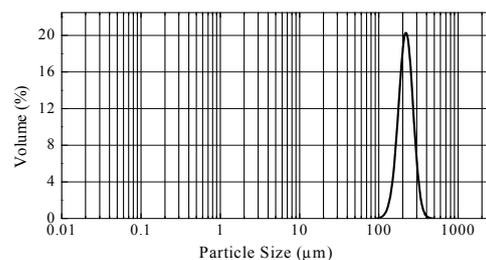
**Figure 1.** Particle size distribution of sand sample
