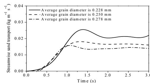
**Figure 8.** Evolution of the streamwise sand transport on beds of different size distributions
