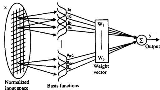
**Figure 1.** Typical structure of a neurofuzzy network (Brown and Harris 1995)
