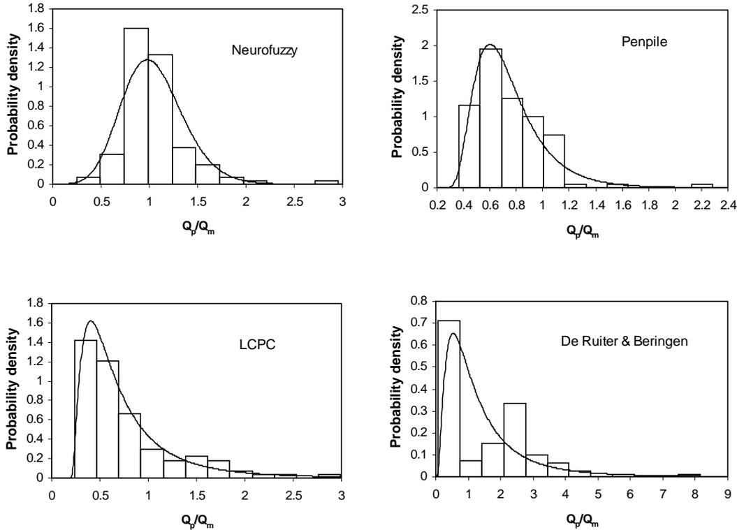
**Figure 4.** Histogram and lognormal distribution curves of  $Q_p/Q_m$  of the pullout capacity methods
