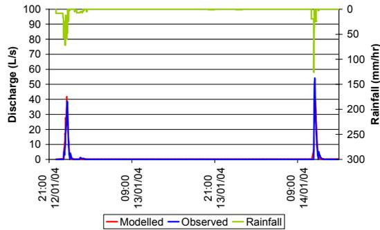
**Figure 4:** Validation hydrograph for the January 2004 event comparing observed and modelled discharge.
