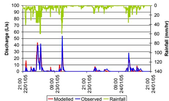
**Figure 3:** Calibration hydrograph for the January, 2004 event comparing observed and modelled discharge.
