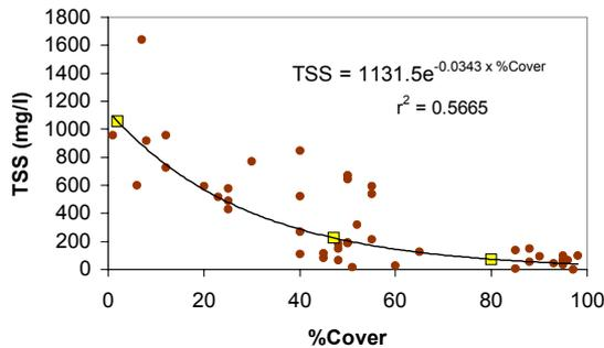
**Figure 8:** Percent cover versus total suspended sediment concentration (TSS) based on microplot data (Roth *et al.*, 2003). Yellow squares indicate predicted concentrations for our 3 patch types.
