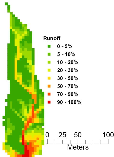
**Figure 5:** Proportion of discharge from each grid cell contributing to the total discharge at the flume for the January, 2005 event.
