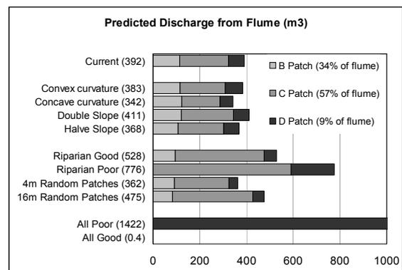
**Figure 1:** Modelled runoff from a 1.2 ha flume for a 230mm rainfall event in January, 2005. B, C and D patches represent good, medium, and poor condition respectively.
