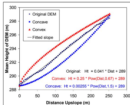
**Figure 6:** Adjustment of DEM to produce convex and concave curvature
