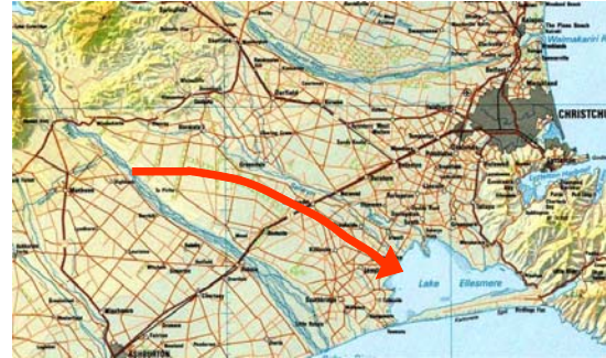
Figure 1. Central Canterbury Plains, New Zealand, showing a typical groundwater flow path provided by the groundwater flow model
