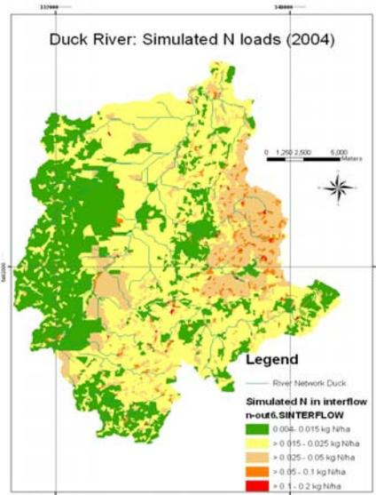
**Figure 9:** Simulated N loads by interflow and stream network for the Duck catchment (2004)
