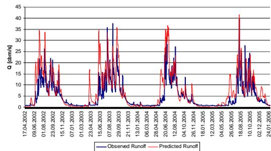
**Figure 4:** Observed and predicted runoff for the Duck Catchment (Year 2002-2005)
