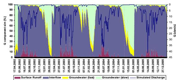
**Figure 6:** Simulated discharge and relative contribution of flow components for the Duck catchment (Year 2002-2006)
