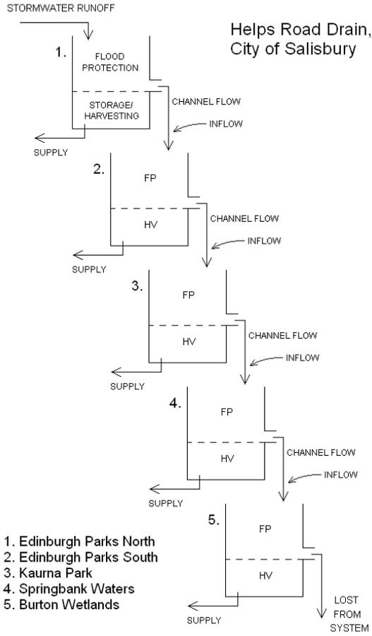
**Figure 1.** Diagram of the Helps Road Drain urban stormwater harvesting system
