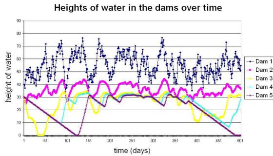
**Figure 4.** The levels of water in the dams over time tend to become smoother further downstream
