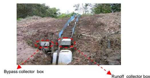
**Figure 4:** Runoff and bypass water collection on canal embankment
