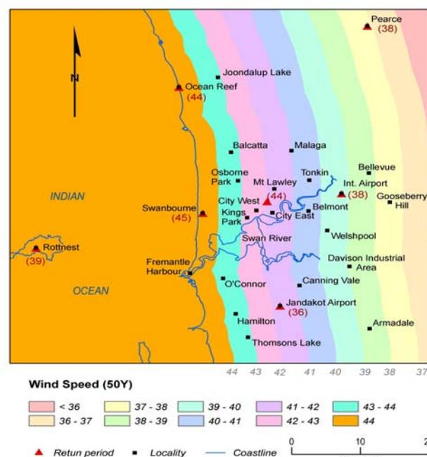
**Figure 2.** Interpolation of 50-yr return-period wind speeds (m/s); open terrain, 10m height, Perth region.
