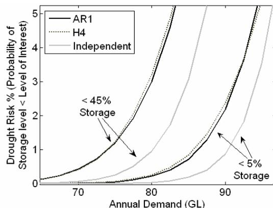
**Figure 10** Simulated long-term drought risk for a reservoir with a capacity of 477.63 GL
