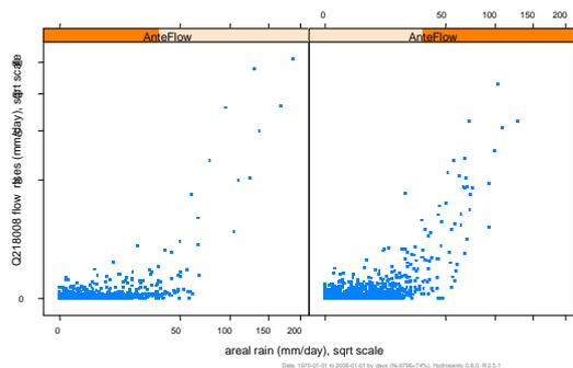
**Figure 8.** Rainfall-runoff relationship showing flow rises at site 218008 as a function of areal rainfall over its catchment, lagged by 1 day. The panels show subsets of the data based on antecedent flow (left panel has days with lowest half of antecedent flows, right panel has the rest).
