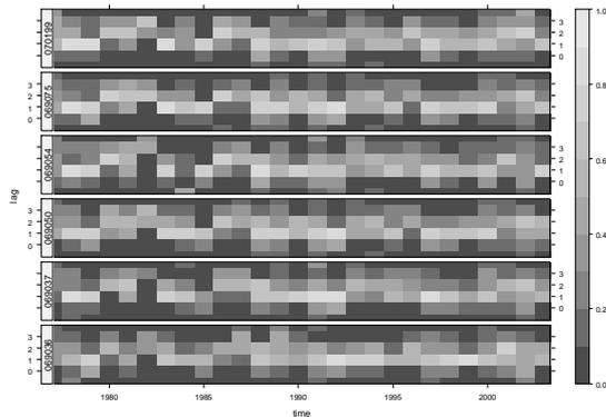
**Figure 5.** Time series of cross-correlation between each of six rainfall series and stream flow rises, aggregated into years. The lag (in days) is marked white where correlation with flow rises is strong.
