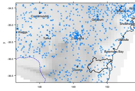
**Figure 3.** Navigating the Australian Daily Rainfall Database. Sites were considered acceptable if they had 10 years of data in the period 1970-2006, and are shown as circles. The Tuross catchment boundary is overlaid. Shading shows elevation interpolated from sites.
