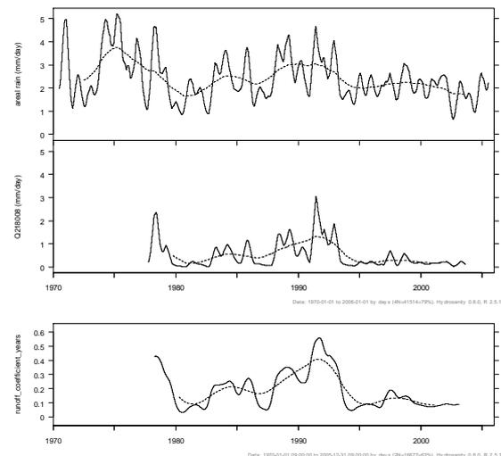
**Figure 7.** Time series of catchment areal rainfall (top), stream flow (middle) and their ratio over a one-year window, the runoff coefficient (bottom). Each series is smoothed with (triangular) kernels of width 1 year and 5 years.
