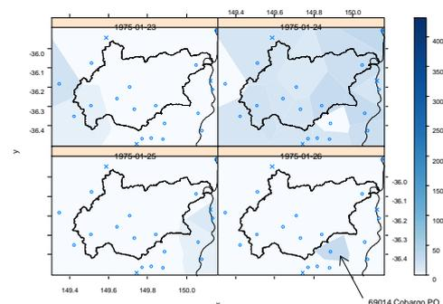
**Figure 2.** Spatial mosaic of rain gauge data, showing a sequence of four time steps (days). A likely timing error presents itself, at site 69014.
