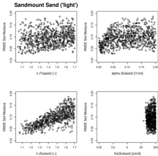
**Figure 3.** Scatterplot relationship between model parameters and RMSE of the soil moisture predictions from 10,000 Monte Carlo simulations (Latin Hypercube sampling) using HYDRUS-1D. Each dot represents a single model realization and its corresponding RMSE.
