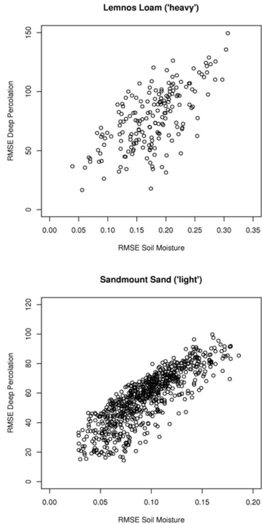
**Figure 4.** Scatterplot relationship between RMSE of soil moisture and deep drainage predictions from 10,000 Monte Carlo realisations with Latin hypercube sampling using HYDRUS-1D. Each dot represents a single model realization and its corresponding RMSE.
