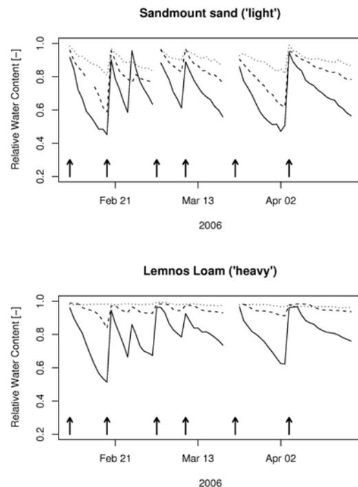
**Figure 2.** Time series of relative water contents (i.e. water contents normalised by maximum water content measured in a particular depth) measured by TDR for selected soil depths: 0.1 m (solid line), 0.3 m (dashed line) and 0.6 m (dotted line).
