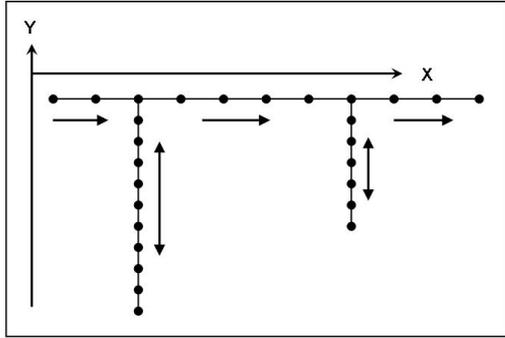
**Figure 1.** Schematic of the channel random walk model with possible diversion to the sub-channel hyporheic zone. Channel particles step from left to right in the  $x$  direction, with chance diversion at right angles from the channel nodes. Two possible diversions of a single random walk are shown.
