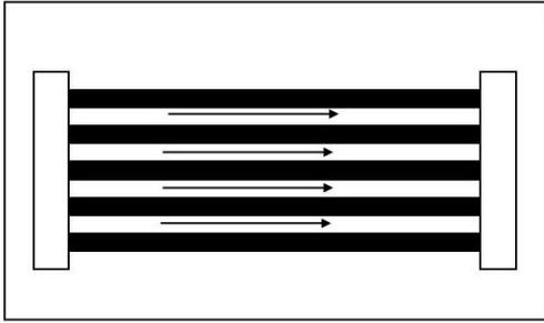
**Figure 5.** Schematic of isolated parallel stream tubes where contaminants are introduced at a vertical input surface on the left and emerge at a vertical mixing surface on the right (after Rasmuson, 1985).
